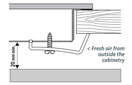
Fig. 1 Thermal protection barrier
